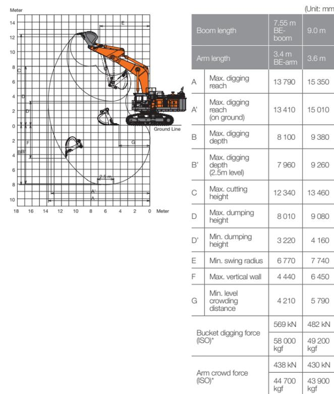
\*This is the calculated value at the loading point (Cutting Edge) conforming to ISO.
